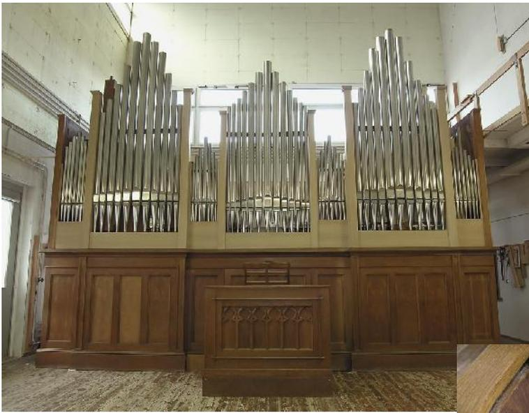
Above is the organ reconstructed with new pilasters to represent the potential casework in the Männedorf workshop. In the course of the reconstruction the instrument was found to be in amazingly good condition, the high quality of the original workmanship clearly demonstrated. Pipework, frames and chests, seen in the following photos, are all substantial and true.
